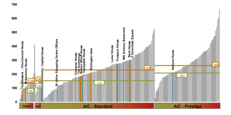
**Figure 2**Energy intensity: Whole building offices – adjusted kWhe/m<sub>2</sub>/yr
